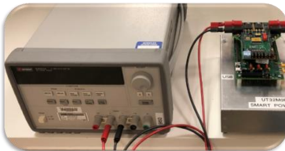
Figure 12: Connect Power Supply to VIN Banana Jacks on SPSC-EVB-R0
