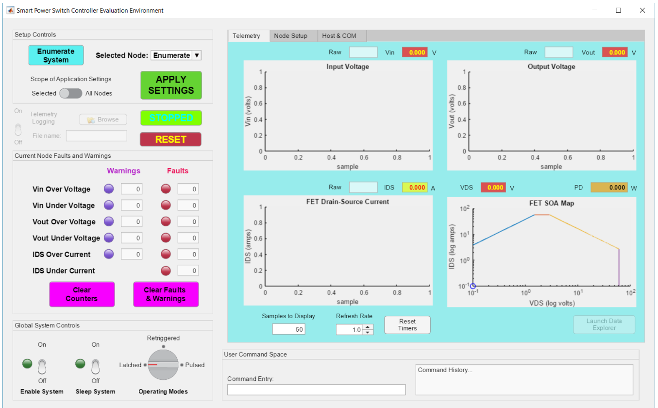
Figure 15: SPSC-EVB-R0-GUI Startup Screen
