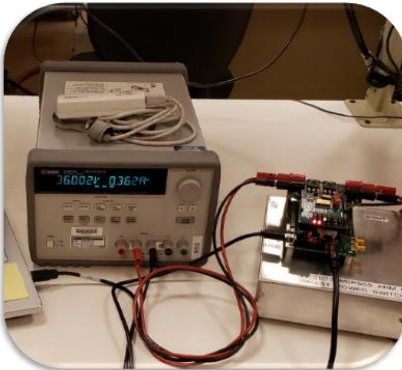
Figure 14: Turn on Power Supply and Set to Desired Voltage
