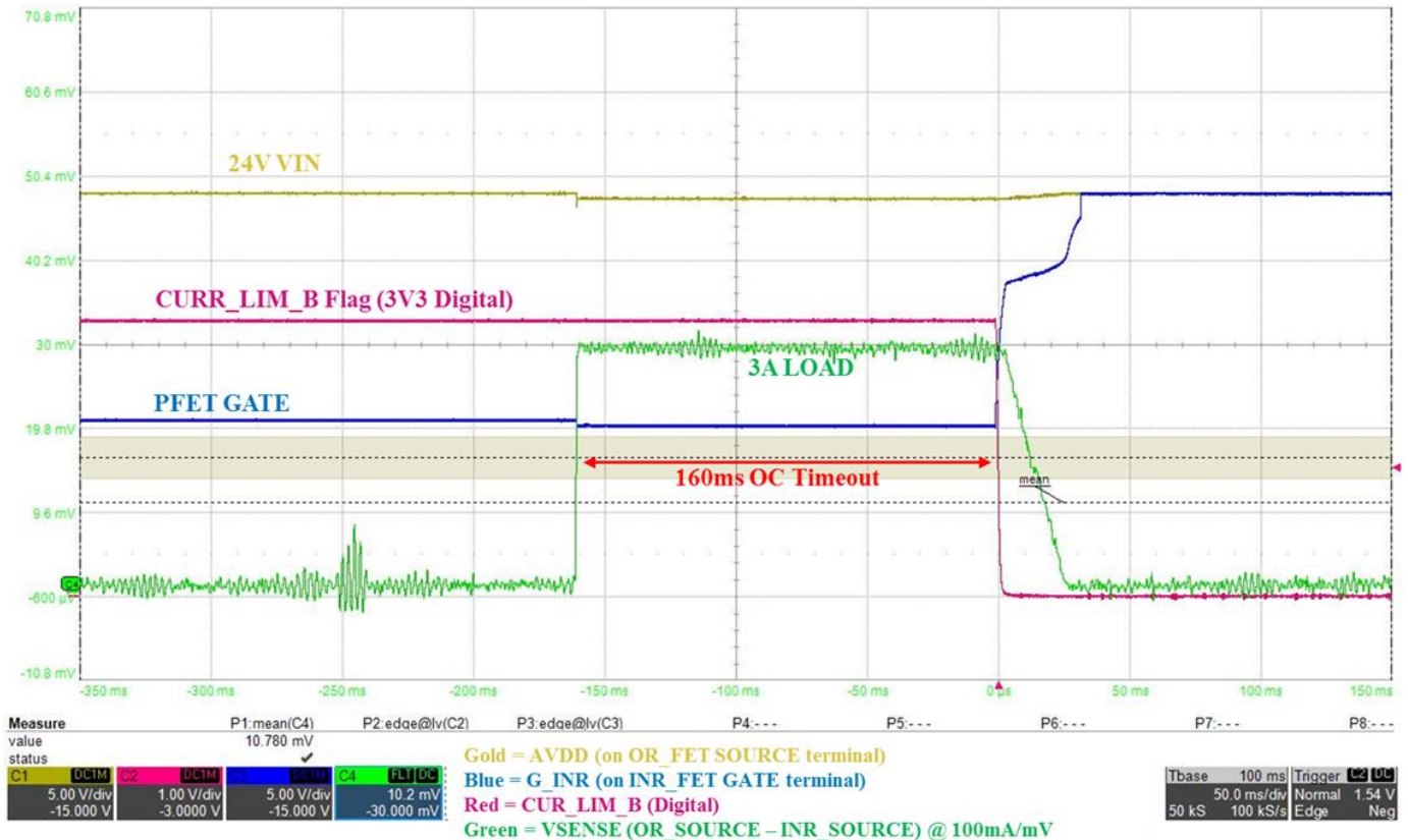
Figure 10: SPSC-EVB-R0 Overcurrent Fault Response
